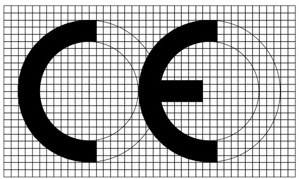
The background-grid should be considered only as an aid and is not part of the CE-marking. If reduction or enlargement of the CE-marking is necessary, the proportions given by the above background-grid shall be followed. The height of the CE-marking should not be less than 5 mm.
